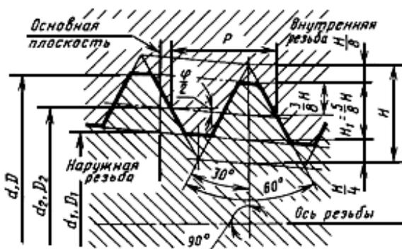
$$\text{Конусность } 2\text{tg } \frac{\varphi}{2} = 1:16; \quad \varphi = 3^{\circ}34'48''; \quad \frac{\varphi}{2} = 1^{\circ}47'24''$$
